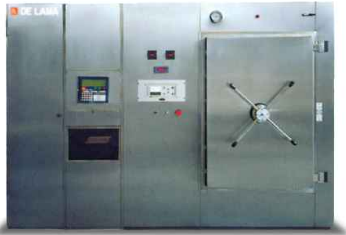
Sterilizer DE LAMA DLOG 541 type , capacity 10875 lts., with hinged door
